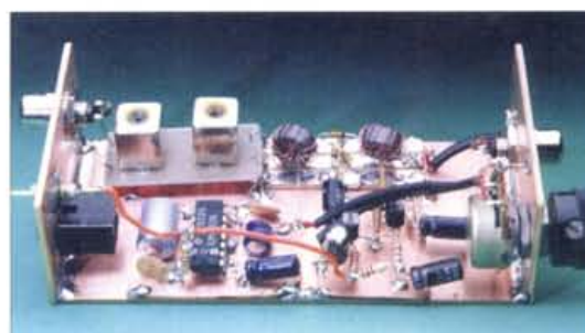
Fig. 1). The signal from the antenna is filtered by a band-pass filter and fed into the DBM. The signal from the Universal VXO, tuning a portion of the 7MHz band, is also fed into the DBM.
