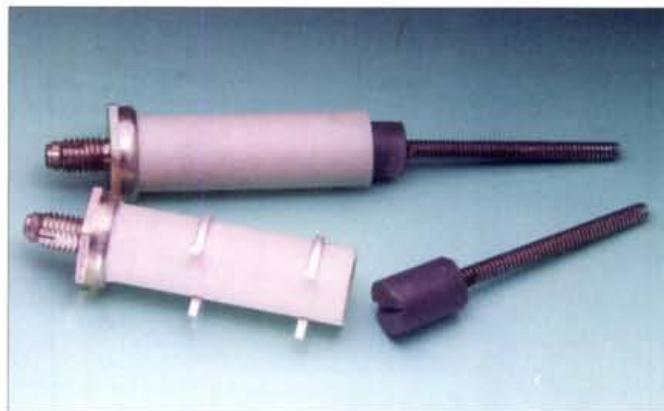
Fig. 2: The high quality (surplus) ceramic coil formers, suitable for use in a 'home-brewed' permeability tuning unit. No fixing nuts are available for the silver-plated threaded ends but G3XFD found that various types fitted and it's thought that the nuts are (or extremely close to) quarter inch UNF types with a thread of 28 turns per inch.
